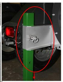
**Important Note**: Stabilizer Leg needs to be put in the down position before un-coupling to insure unit doesn't tip or roll over.
