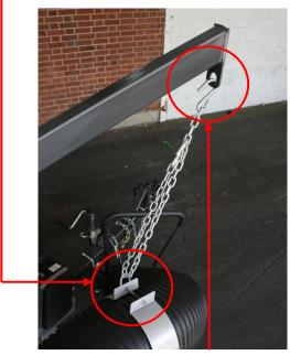
(E) Install Support chain (4') between Hose and Boom
