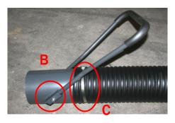
C: Attach Nozzle Assembly to One End of the Intake Hose Utilizing 8" Worm Drive Clamp.
