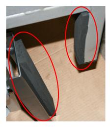
**Note:** Leave clamping plates loose to swivel for easier installations.
